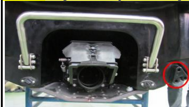
SS316 Boarding Ladder and peed Measuring Device
